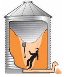
A center grain unloading auger draws grain from the top center and the grain forms a cone as the bin is emptied. Illustration:
