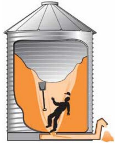
A center grain unloading auger draws grain from the top center and the grain forms a cone as the bin is emptied. Illustration: John A. Kramer, Safety Measures in Handling Stored Grain, Kansas State University, February 1989.
