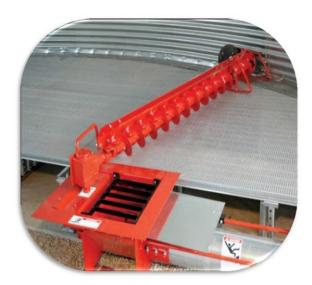
the auger, or a dead-man switch on an operating control inside an enclosure or attached to a handle that keeps the employee seven feet back from the auger); **and** the facility's bin-entry permit procedures are followed.
